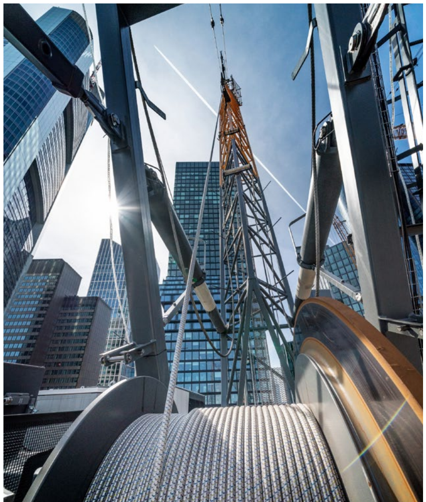
The 258 HC-L 10/18 Fibre crane from Liebherr features a 25 mm fibre rope.
