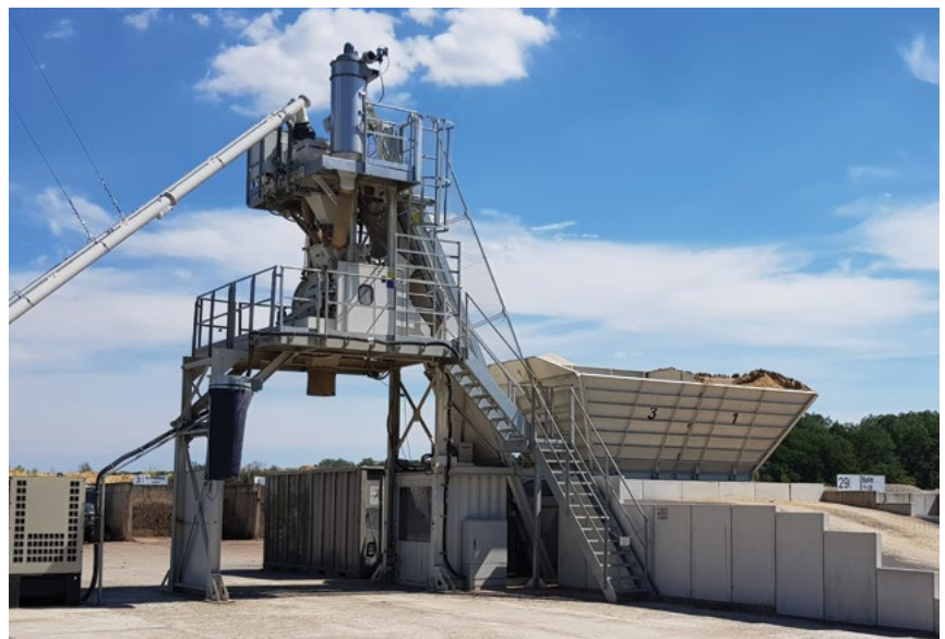
The CBT 60 SL Elba concrete mixing plant.
