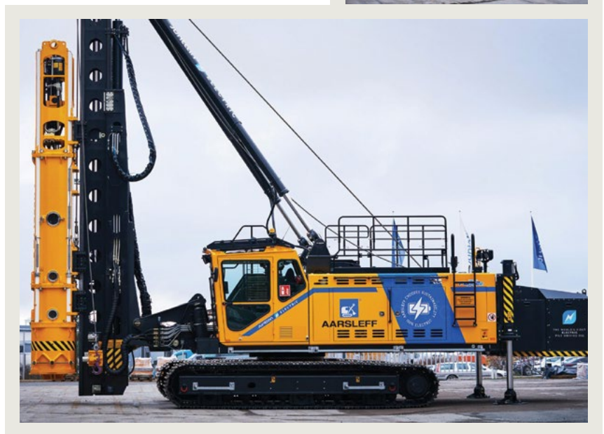
The fully battery-powered eJunttan PMx2e electric pile driving rig.
