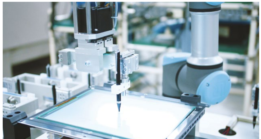
Japan-based Koyo Electronics Industries made a jig that can be used for any stylus patterns required for inspection, by modifying the combination of the UR cobot's end effector.
